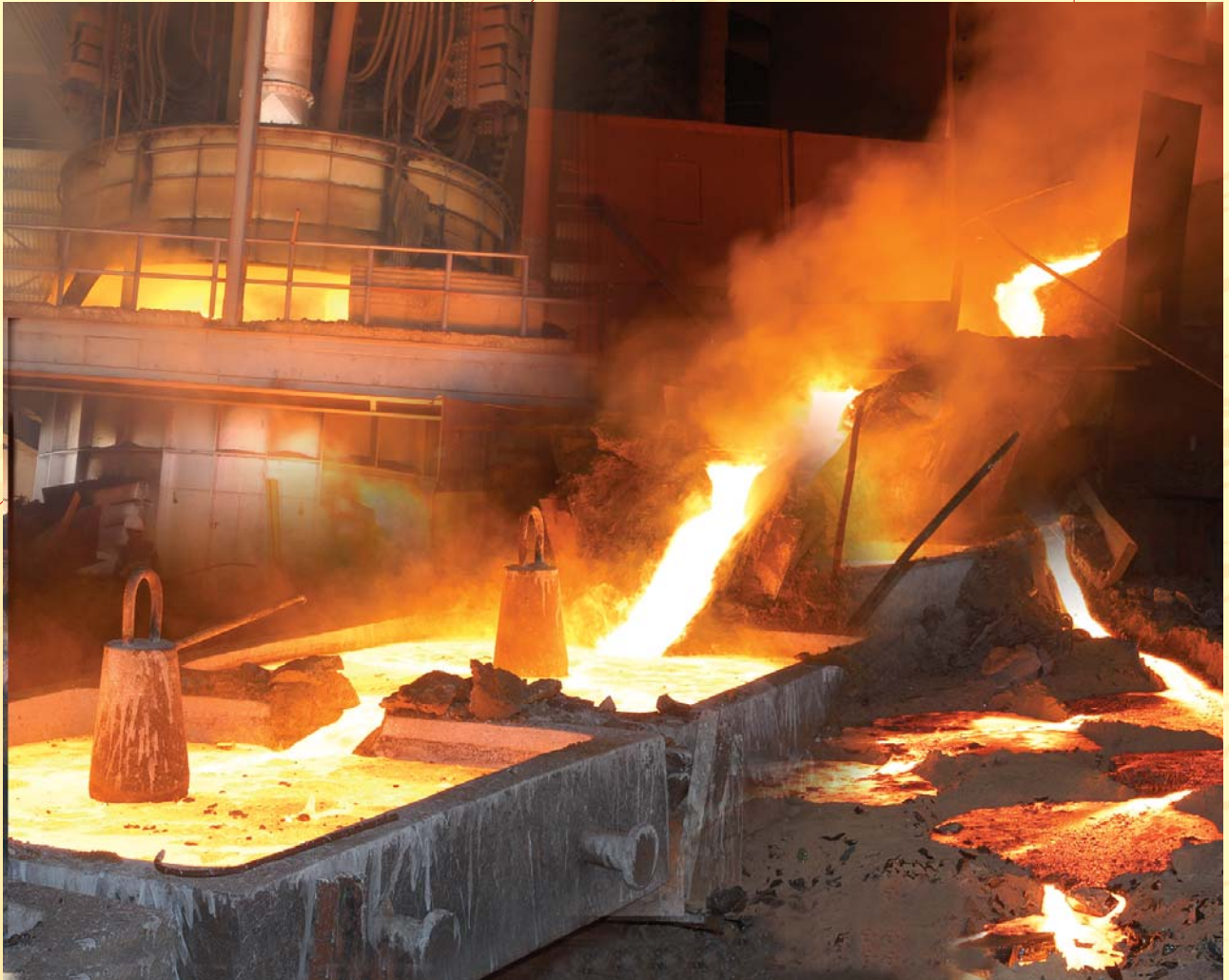
Continuous tapping of Ferro Alloys in Submerged ARC Furnace
